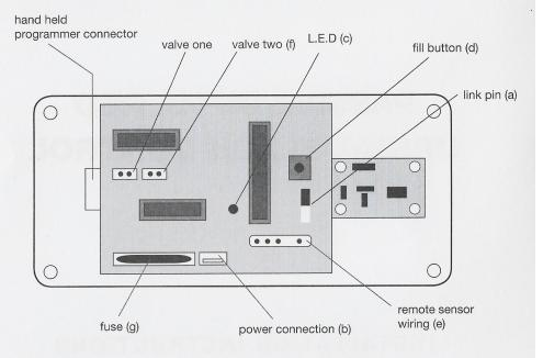
6. Connect the battery pack to the circuit board (marked B on the diagram). Do not allow the battery pack to hang unsupported. This will power up the Greenflow. The LED on the printed circuit Board will give two long flashes followed by two short flashes, indicating that it is ready to set the valve.
